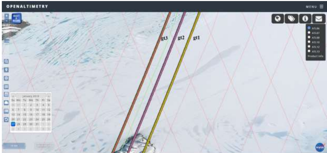
Figure 2: ICESat-2 track-462 over the selected Melt pond showing the beams gt1, gt2 and gt3 on 27/01/2019 from openaltimetry.org for ATL06 and ATL03 datasets
